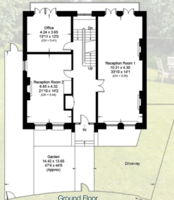
Ground Floor Approximate Area = 116.7 sq m / 1,256 sq ft Including Limited Use Area (0.5 sq m / 5 sq ft)
